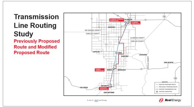
This slide shows the Previously Proposed Route as a blue dashed line and the Modified Proposed Route as a red dashed line. The existing electric transmission line is shown as a black dashed line.
